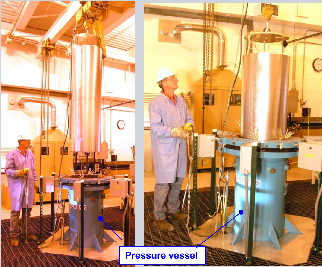
Article lowered into the pressure vessel
